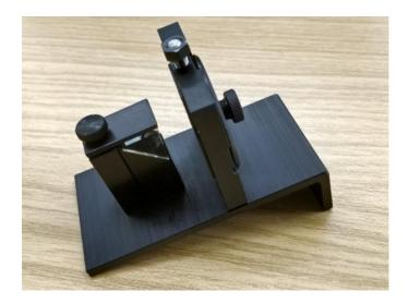
The miniature BLS setup is a compact and complete back-scattering setup that can be used to test a TFP-1 or TFP-2 spectrometer. Being quite small, the setup can be used without removing to the remaining optics surrounding the device.
